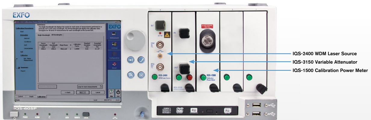
A typical power-measurement setup.
