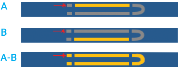
Using the loopback test method and iLOOP option on your iOLM enables you to test two fibers at once. View only the A link, B link, or the complete A-B link including the loop.
